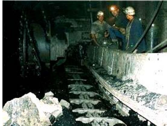
Conveyor installed in main tunnel and underground coal excavation and transportation system (Breza Coal Mines)
