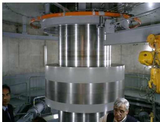
Shaft to Connect Generator and Turbine, Constructed by the Project
