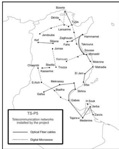
Figure 1 Telecommunication networks installed by the project TS-P5
