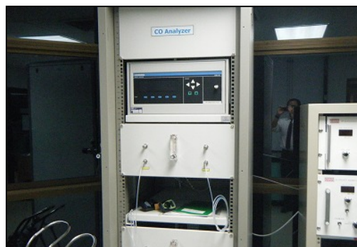
Photo 2: Analysis instrument (NOx, SO 2 , CO, etc.)
