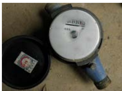
House water meter face blurred with \text{CaCO}_3 in Quang Son, Ninh Binh
