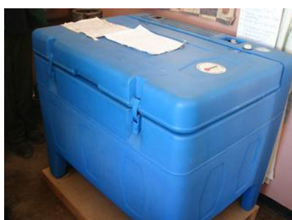
Gas/electric refrigerator (at a missionary hospital in Chongwe)
