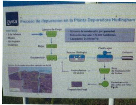
Photo 2 Facility Chart of the Sewage Disposal Plant
