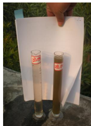
Fig. 6 Before treatment (right) and after treatment (left) (Jiaxing Sewage Treatment Plant)
