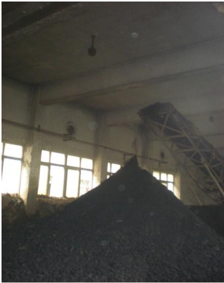
Fig. 12 Sludge with 60% moisture content (Jiaxing Sewage Treatment Plant)
