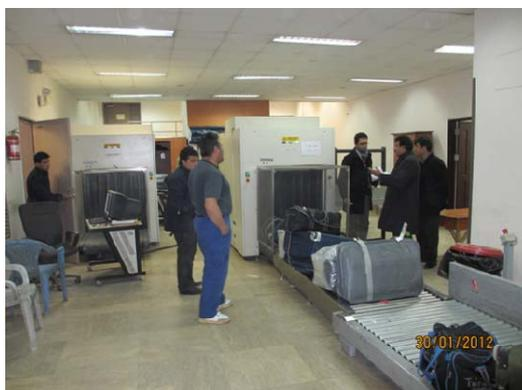
X-ray inspection machine for checked baggage
