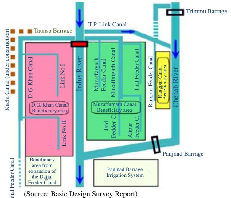
Figure 1: Layout of Irrigation Canals of the Taunsa Barrage
