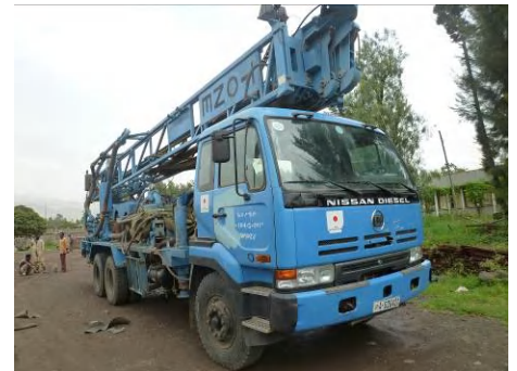
Well Drilling Rig
