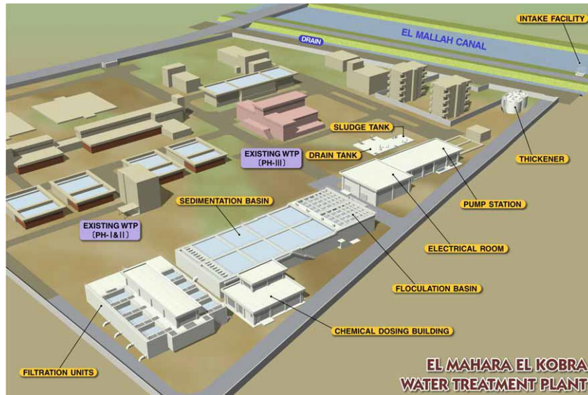
Source: Compiled based on the treatment plant diagram in the Base Design Study Report Figure 2: El Mahala El Kobra Water Treatment Plant of the Project
