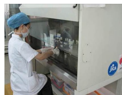
Safety cabinet installed to the infection control laboratory at FAH-GMC
