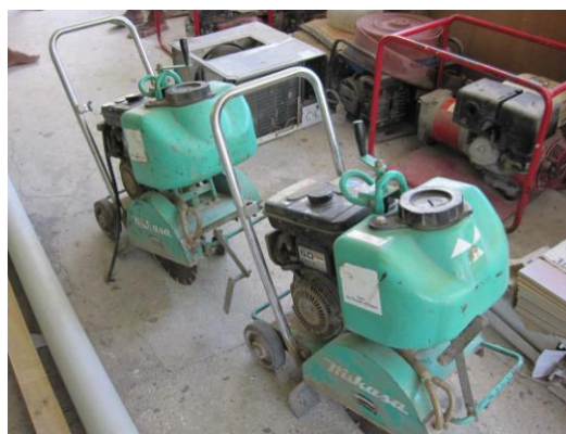
Photo 1: Two Concrete Cutters Provided in the Project
