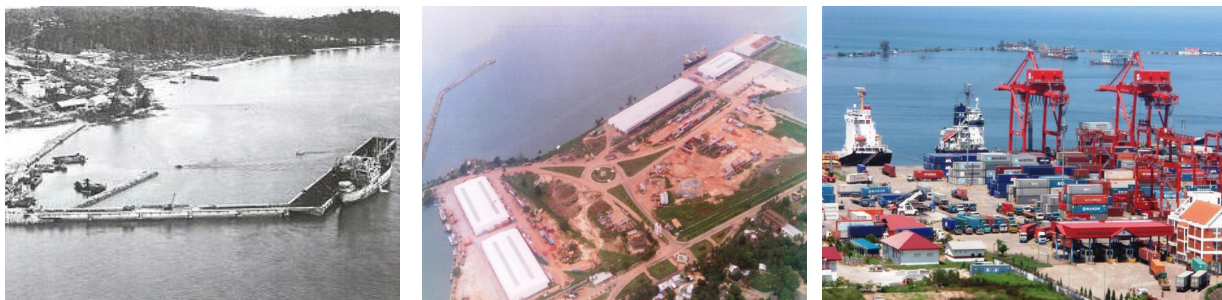
Figure 4: Transitions of Sihanoukville Port Left: At the Time of the Opening of the Port in 1960, Center: Before the Project Implementation in 1996, Right: After the Project Completion in 2011
