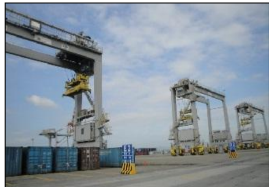
Rubber Tired Gantry Crane
