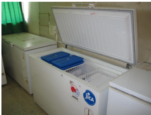
Ice-lined refrigerator provided under this project (Tonga)
