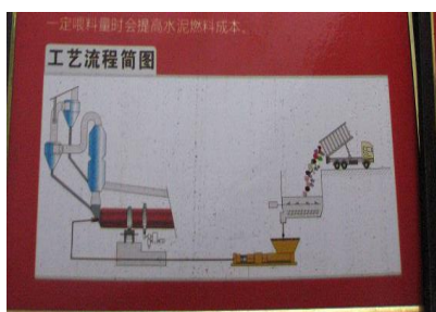
Figure 2: Sludge Recycling Process Chart Displayed at the Plant
