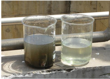
Figure 1: Pre-treatment water (left) and treated water (right) at the Linjiangxi Sewage Treatment Plant
