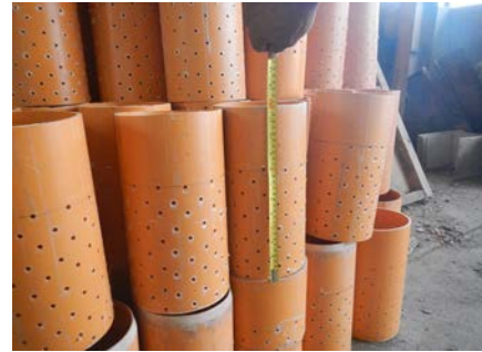
Figure 13: Perch Tubes (used to adjust paddy field water)
