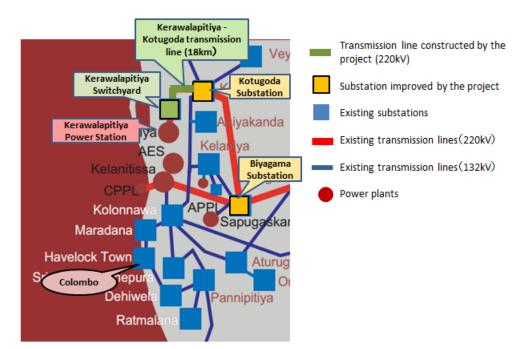
Figure 2 Location of the Facilities Constructed by the Project
