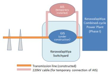
Figure 3 Extension of 220kV cable for temporary AIS
