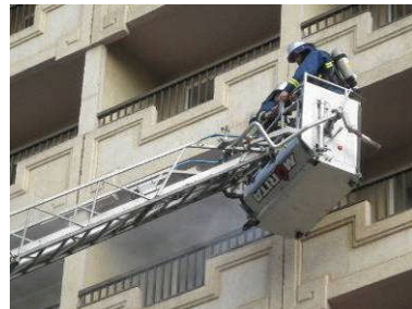
Basket at the top of ladder
