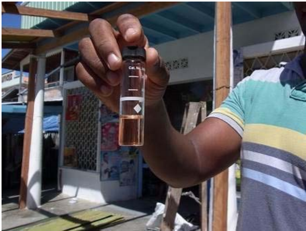
Checking of the iron concentration using a reagent (in an area receiving untreated water)
