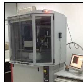
Single-crystal X-ray diffraction spectrometer. Operating for almost 24 hours a day. Kept in good conditions with maintenance by a teacher and a graduate student. (Henan University)
