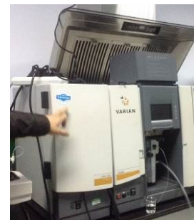
Atomic absorption spectrometer being used for testing of heavy metals in an assessment of industrial hygiene. (Shangqiu Normal Univ.)
