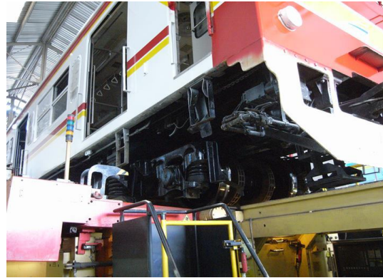
Photo 2. Maintenance of railcars using a wheel tread reprofiling machine
