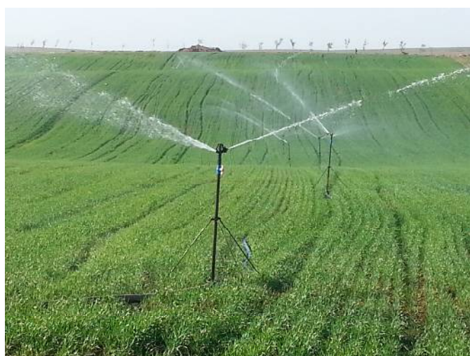
Semi-fixed sprinkler in the model site of Dashixiang in Murei County, the Xinjiang Uygur Autonomous Region
