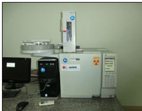
A gas chromatograph (GC), which measures the content of various components in a sample, and accessories supported by the “Technology Project”
