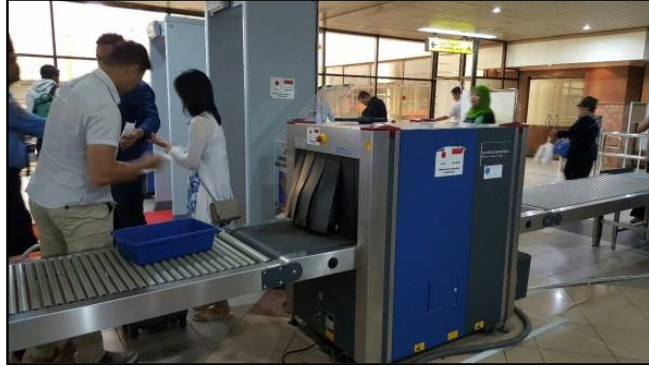
Procured X-ray machine & walk-through metal detector in Batam Airport
