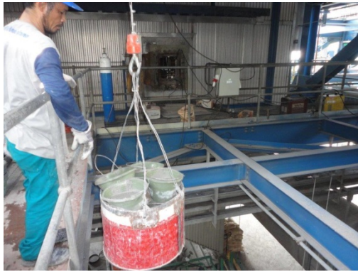
A Staff Bringing Combustion Mediator (Silica Sand) which is Used for CFB Boiler
