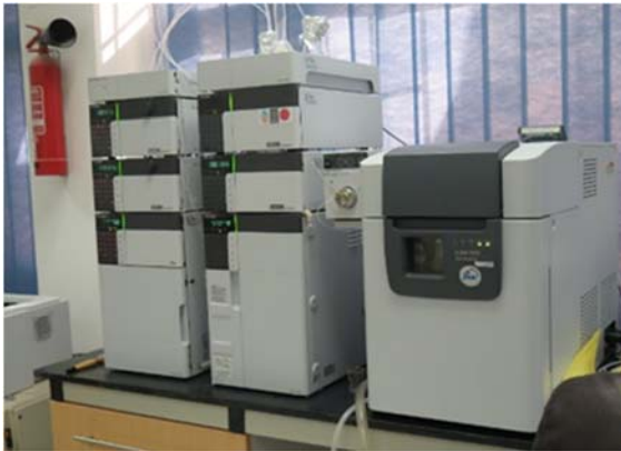
Liquid chromatograph capable of high performance mass spectrometry
