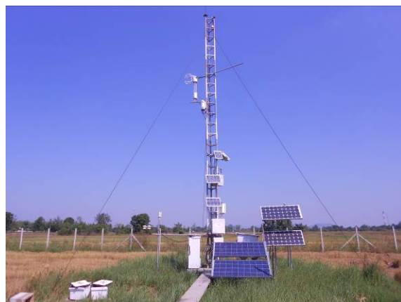
Photo 1: Flux observation tower installed in Ratchaburi
