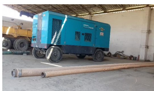
Procured drilling compressor
