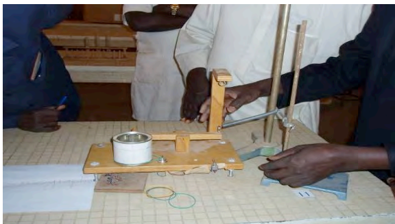
A teaching material for a laboratory experiment in geoscience developed by the project (seismograph)
