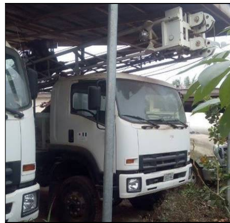
Truck mounted drilling rig
