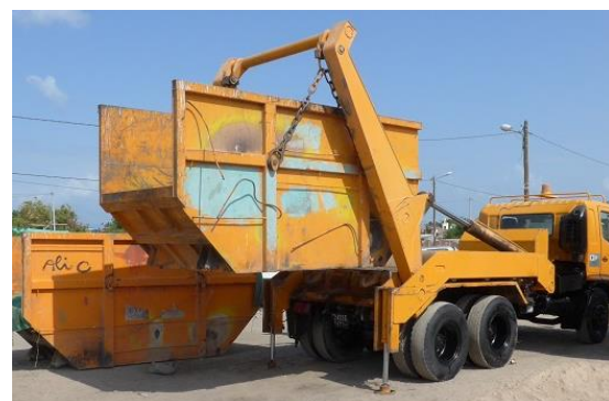
A container truck (10 m 3 ) with broken sidebars
