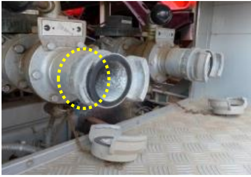
Corroded areas in hose connection parts
