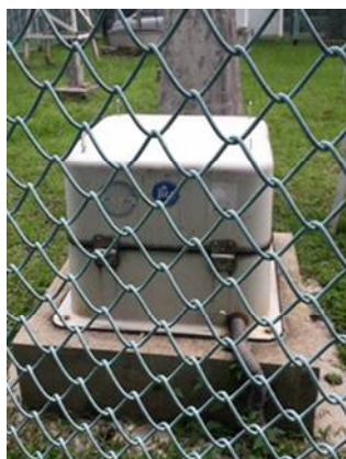
Fixed Accelerometer installed at front yard of Life Science Faculty, ITB
