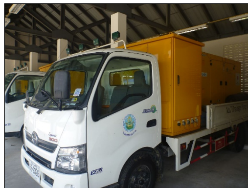
Photo 2: Drainage Pump Vehicle
