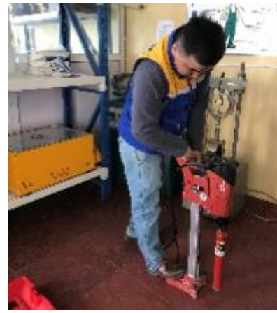
Core drilling machine provided by the project
