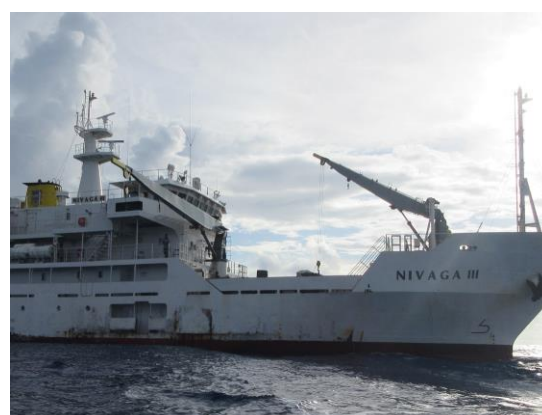
Side of the ship body (rusts and paint peeling)
