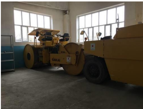
A road roller (left) / a tire roller (right)
