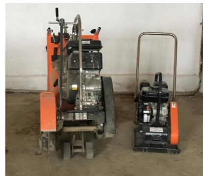
An asphalt cutter (left) and a vibration compactor (right): the most installed equipment
