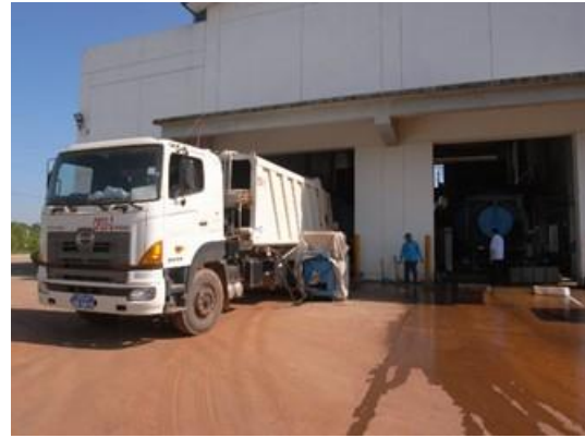
Photo 3. Same as left (Transshipment of waste to a large (20m 3 ) compactor truck that transports waste to the final disposal site)
