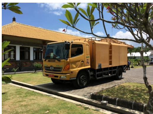
Photo 1: Cleaning Vehicle Procured in This Project (Water jet cleaner)
