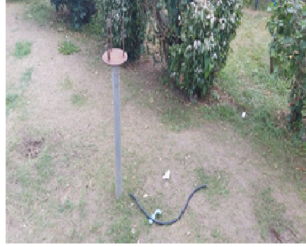
Water gauge damaged by heavy rain in Tamboko Village
