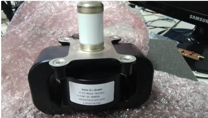
“Magnetron” is a new purchased spare part for the X-Band Doppler Radar that attached to the Mobile Parameter Radar”
