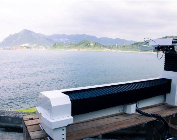
Photo 2 (provided by MMU): MMU utilized the SAR sub-system for further development of a ground-based SAR (GBSAR) to detect land deformation. According to MMU, GBSAR has higher detection accuracy compared to CP/SAR and can detect sub-mm movement on natural or synthetic objects.
