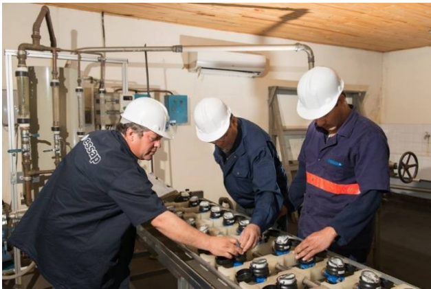
Training on accuracy verification of water meters
