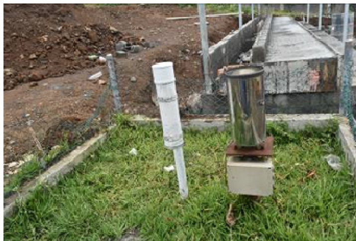
Rain gauge at Quatres Soeurs, installed by Mauritius Meteorological Services as a complementary tool for the MPI's monitoring system
