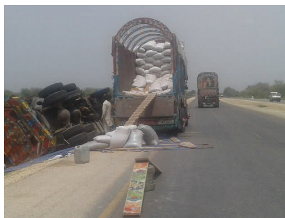
Photo 4: Accident Caused by Overloading
