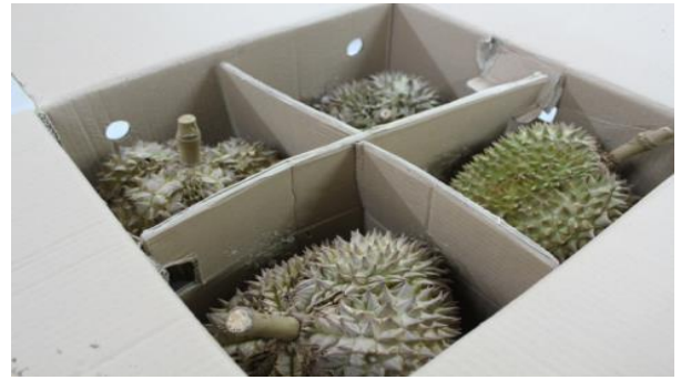
Corrugated carton box: Transport packaging for fresh durian developed by the project
