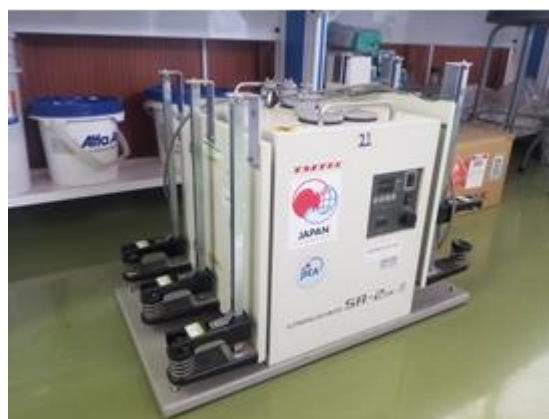
Vertical shaker for sample preparation
