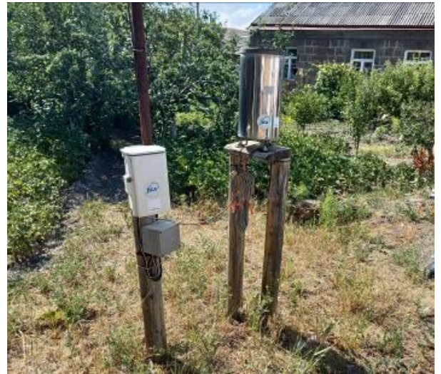
A set of tipping bucket rain gauge provided by the project also maintained in good condition (in Arapi)
