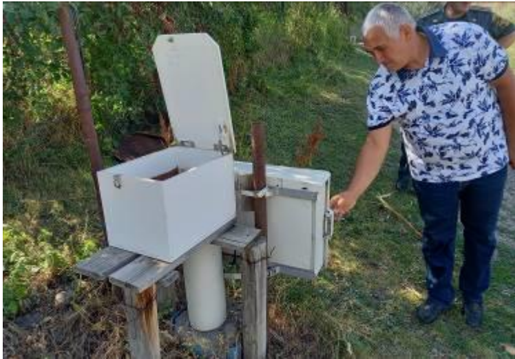
An MES engineer checking the operational status of landslide monitoring equipment provided by the project (in Arapi)
